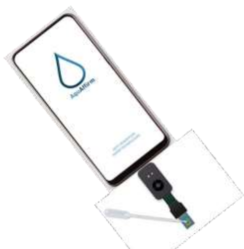
AquAffirm™ smartphone-based platform for water contaminant testing.
